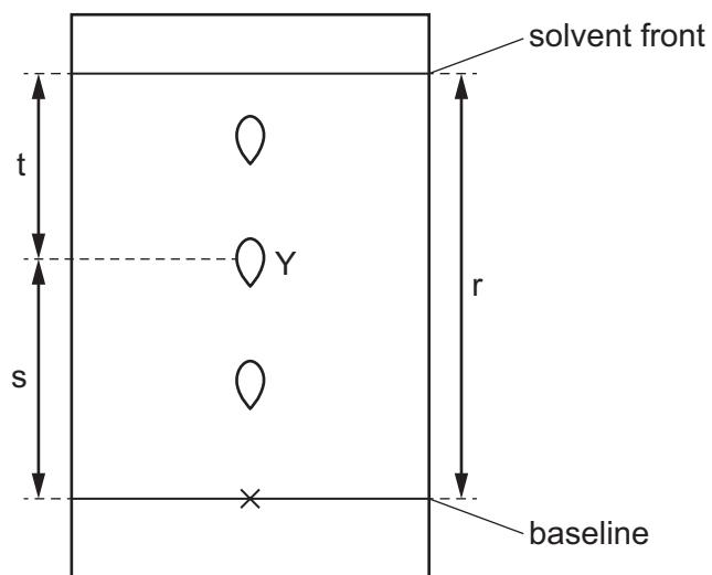
How is the  $R_f$  value of substance Y calculated?
