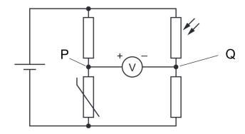
One way to approach this question is to consider the p.d. across P and Q indicated on the circuit diagram. As the temperature increases, the resistance of the thermistor decreases and the p.d. across the thermistor falls – the voltmeter reading will decrease. As the light intensity increases, the resistance of the light dependent resistor (LDR) decreases and the p.d. across the LDR falls – the voltmeter reading will again decrease. Answer **A**.
