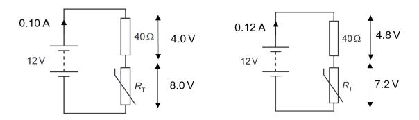
Initially, the current in the circuit is 0.10 A, so the p.d. across the fixed resistor is 4 V and the p.d. across the thermistor is 8 V.
