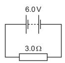
How much energy is transferred in the 3.0  $\Omega$  resistor in 30 seconds?
