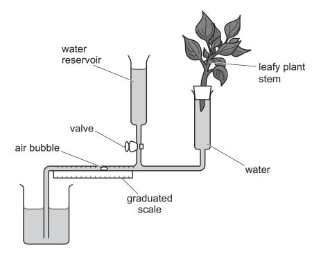
The cut end of a leafy plant stem is inserted in the apparatus. As transpiration occurs, water moves up the stem and is absorbed. This causes the air bubble in the apparatus to move along the tube towards the stem. The distance moved by this bubble in a known time is a measure of the rate of transpiration.
