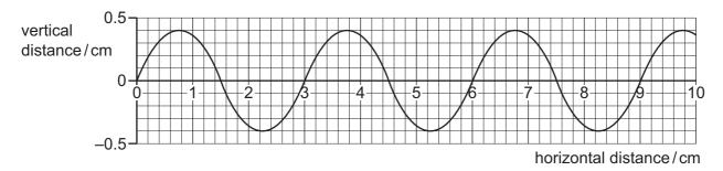
Which row gives the wavelength and amplitude of this wave?
