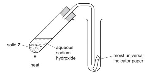
When the test-tube is heated, the indicator paper turns blue.
