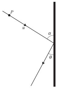
A particle P of mass m is moving with speed u on a fixed smooth horizontal surface. It collides at an angle  $\alpha$  with a fixed smooth vertical barrier. After the collision, P moves at an angle  $\theta$  with the barrier, where  $\tan \theta = \frac{1}{2}$  (see diagram). The coefficient of restitution between P and the barrier is e. The particle P loses 20% of its kinetic energy as a result of the collision.
