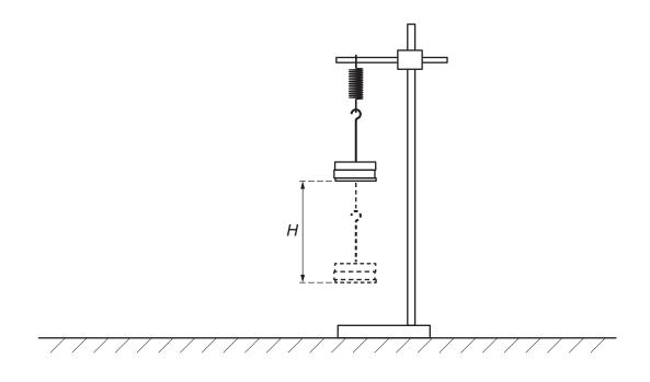
• The distance between the lowest and highest positions of the oscillating mass hanger is *H*, as shown in Fig. 2.3.
