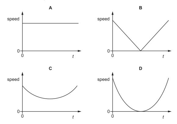
7 A train, initially at rest at a station, has a uniform acceleration of  $0.20 \,\mathrm{m\,s^{-2}}$  until it reaches a speed of  $20 \,\mathrm{m\,s^{-1}}$ . It travels for a time at this constant speed and then has a uniform deceleration of  $0.40 \,\mathrm{m\,s^{-2}}$  until it comes to rest at the next station. The distance between the two stations is  $3000 \,\mathrm{m}$ .
