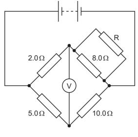
The voltmeter reading is zero.
