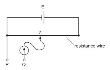
Z is a connection that may be made at any position along the resistance wire. A galvanometer is connected between Z and a point Q.
