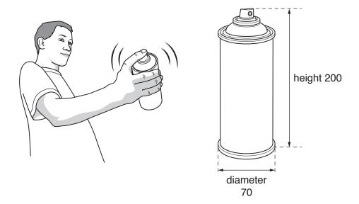
Design a device that will shake a spray paint can so that the contents are mixed well.
