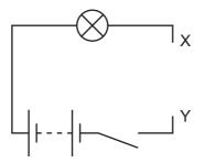
The student wishes to connect a component between X and Y to enable her to vary the brightness of the lamp.
