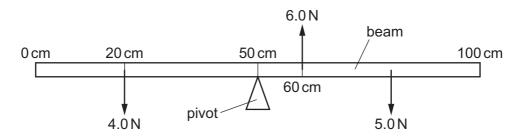
The beam remains balanced on a pivot at the 50 cm mark under the action of the forces of 4.0 N, 5.0 N and 6.0 N.
