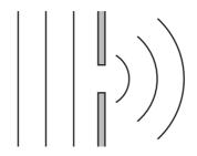
The waves approach a barrier and pass through the gap in the barrier.
