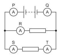
Which statement about the readings on the ammeters is **not** correct?
