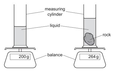
Which two measurements does the student need to make to determine the density of the rock?
