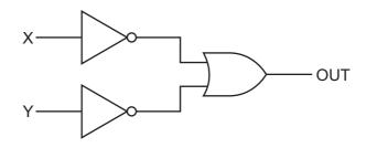
Which single logic gate, placed between X, Y and OUT, would have the same effect as the network?
