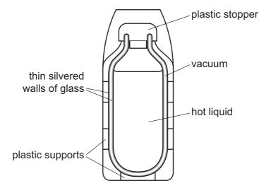
Which methods of thermal energy transfer are the silvered walls designed to reduce?
