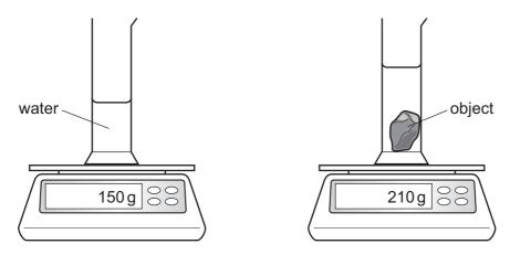
A solid object is put in the cylinder and the water level rises to  $75\,\text{cm}^3$ .
