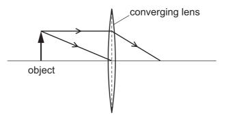
An image of the object is formed on a screen to the right of the lens.
