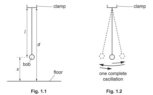
(a) The student measures the distance *d* between the bottom of the clamp and the floor.
