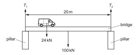
The pillars exert forces  $T_1$  and  $T_2$  on the ends of the bridge.
