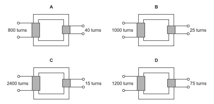
**36** Which transformer can change a 240 V a.c. input into a 15 V a.c. output?
