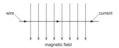
The magnetic field causes a force on the wire.
