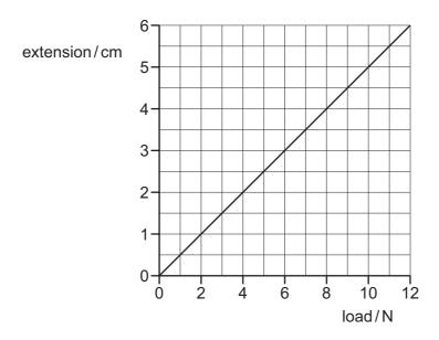
A load is hung from the spring and the length of the spring increases to 5.0 cm.
