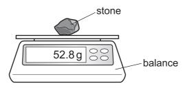
The stone is lowered carefully into a measuring cylinder that contains 50 cm<sup>3</sup> of water. The level of the water in the measuring cylinder rises to the 72 cm<sup>3</sup> mark.
